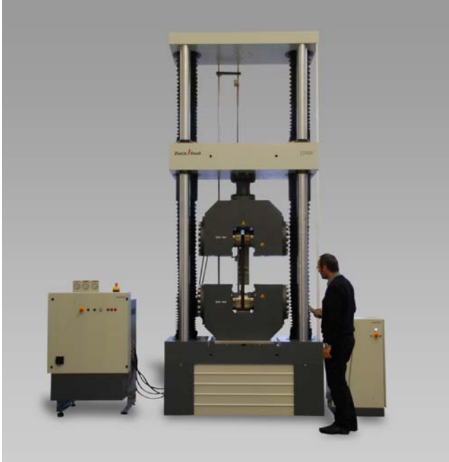
Figure: Zwick Z2000E with hydraulic grips
